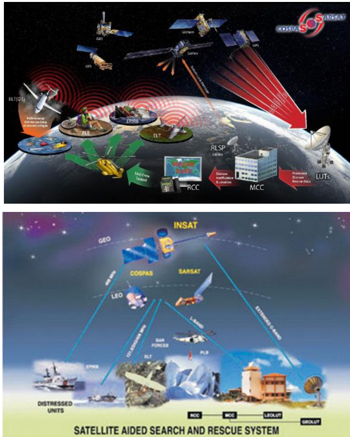
Overall system configuration of COSPAS-SARSAT (from https://earth.esa.int/web/eoportal/satellite-missions/c-missions/cospas )
